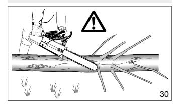
Start limbing by leaving the lower limbs to support the log off the ground (fig. 30). Always cut from the top of the limb. Do not underbuck freely hanging limbs. A pinch may result or the limb may fall, causing loss of control. If a pinch occurs, stop the engine and remove the saw, by lifting the limb.
